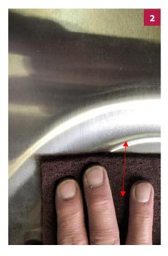
Continue rubbing until the surface is free of minor scratches or scuffs. Widen the area to blend between the manufactured and repaired finish.
