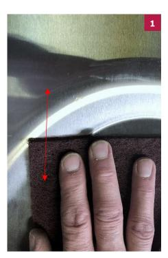
Identify minor scratches or scuffs. In the same direction of polished finish, rub in-line with a marron *Scotch-Brite*<sup>™</sup> finishing pad over the damaged area.
