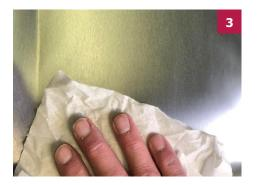
After blending. Rub the entire surface with a stainless-steel wipe or cleaner solution and a soft cloth to create an even finish.
