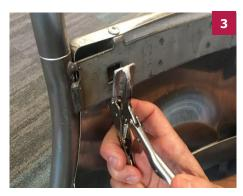
Hold in place with clamp bottom ("U" shaped section).
