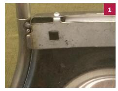
Remove broken or malfunctioning stud retainer assembly. **Note:** Upper retainer assembly is not used for Non-Upholstered (Vision-NU) seat backs.
