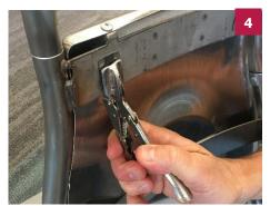
Position top of stud retainer assembly (two parts, see next image) and firmly clamp together to secure.
