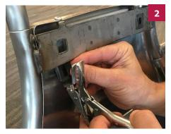
Position one stud retainer bottom behind the back strap and lined up with the openings. (AmSeCo part number: 114880000)
