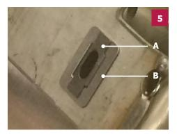
Repaired stud retainer. Item A is the stud retainer upper and item B is the guard. (AmSeCo part numbers A: 114879000 and B: 155451500)
