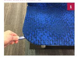
Starting at the front side edges of the seat cushion onsert, slide a pry tool between the onsert and the seat frame and rotate.
