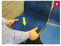
Next, firmly depress the two serrated studs into the retainer assemblies of the seat module. Audible clicking will be heard, push down until clicking stops.
