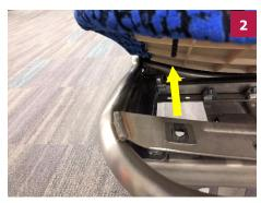
Then, pry away the seat cushion onsert to release two serrated studs from the retainer assembly at each corner.
