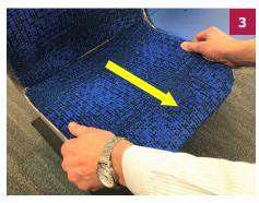
Pull the onsert forward to disengage the two washer heads from the smaller opening of the keyway slots in the seat module, then pull the seat onsert upward to remove out of the larger opening.
