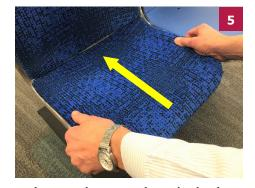
Push rearward to engage the washer heads to the back (smaller opening) of the keyways, be sure that the back of the seat is touching the bottom of the back.
