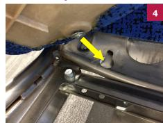
Insert the two washer heads into the larger openings of the keyways on the seat module.
