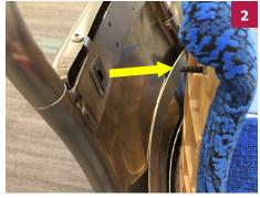
Then, pry away the back onsert to release two serrated studs from the retainer assembly at each corner.
