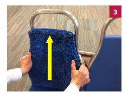
Next, lift the back onsert up to disengage the bottom two washer head bolts from the keyways on the seat module.
