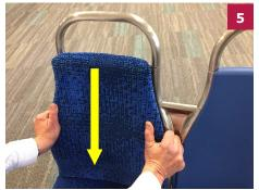
Then, push down to engage the washer heads into the smaller openings of the keyways.
