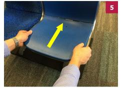
Push rearward to engage the washer heads to the back (smaller opening) of the keyways, be sure that the back lip of the seat tucks under the bottom of the back.
