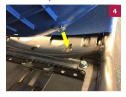
Insert the two washer heads into the larger openings of the keyways on the seat module.
