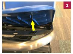
Then, pry away the seat cushion onsert to release two serrated studs from the retainer assembly at each corner.
