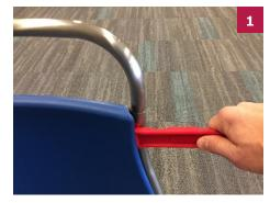
Starting at the upper side edges of the seat back, slide a pry tool between the onsert and the seat frame and rotate.
