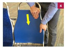
Replace the back before the seat. Bring the back close to the final location but start about 1 - 2 inches high so the middle spring clips are above the strap (see 5).
