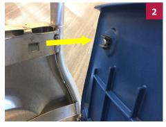
Then, pry away the back onsert to release two spring clips from the square opening at each corner. Reference image only, the back onsert will still be close to frame (3).
