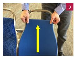
Next, lift the back onsert up to disengage the mid-section spring clips behind cross member strap of the seat module. This a little tricky as the clips are under tension.
