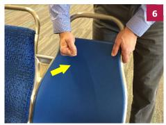
After the middle clips are engaged, align the square clips to the square openings (see 2) and tap the onsert from the front to insert the clips into openings.
