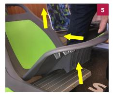
The weight of the seat module will fall back, but removal is up, back and up.
