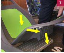
Hook the new seat over the back of the extrusion and rotate forward and down.
