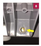
Align mount and extrusion rivet-nut holes, picture shows slight misalignment.
