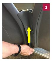
Push (bend-twist) the seat-tie up and remove from between transverse seats.
