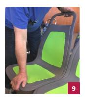
Pull the grab handle forward and push down on the front edge of the seat.
