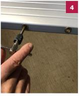
Clean out both rivet-nut threads with a 5/16"-18 thread tap.
