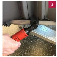
Remove the seat tie bolt from the back of the extrusion with a T30 TORX bit.
