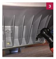
Remove the two seat bolts from the front of the extrusion mount area.
