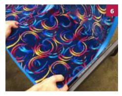
Firmly depress the two serrated studs into the seat module. Audible clicking will be heard once the studs enter the retainer assembly. Push down until clicking stops.
