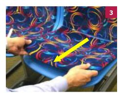
Next, pull the seat onsert forward to remove the two spring clips from the slots in the seat module.
