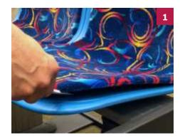
Starting at the front corners of the seat, slide the tapered end stick between the onsert and the seat module and lift.
