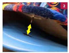
Then, pry up the seat onsert to release the two serrated studs from the retainer assembly at each corner.
