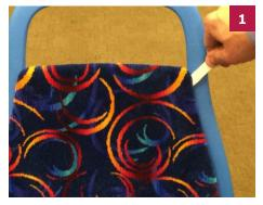
Starting at the top corner of the seat back, slide the tapered end stick between the onsert and the seat module and lift.
