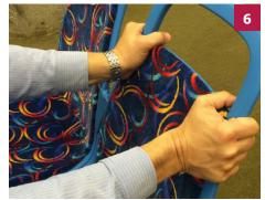
Firmly depress the two serrated studs into the seat module. Audible clicking will be heard once the studs enter the clip assemble. Push down until clicking stops.
