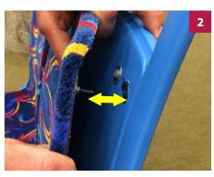
Then, pry up the back onsert to release the two serrated studs from the retainer assembly at each corner.
