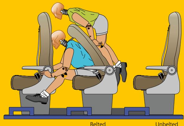
Seating without **SmartFrame** is not designed to provide full compartmentalization, leaving unbelted passengers vulnerable to forward momentum.
