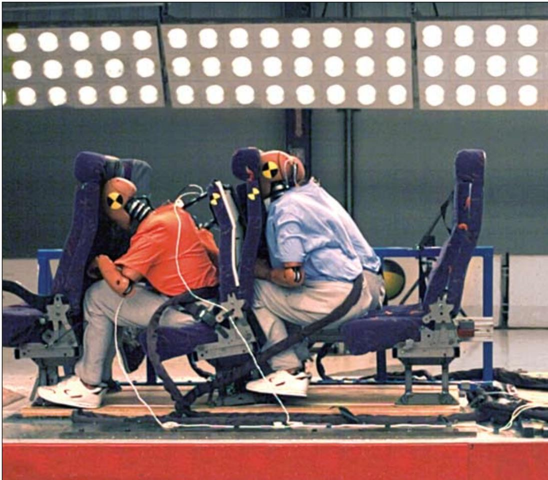
Motorcoach seats by American Seating and SafeGuard<sup>®</sup> undergo the most rigorous testing in the transportation industry. Over the past decade, SafeGuard engineers have conducted twelve full barrier crash tests, more than two hundred sled tests and twenty rollover tests on buses to gain a full understanding of bus occupant protection.
