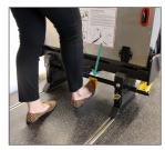
Forward facing pedal: Push down on pedal to release lock and push seat into place
