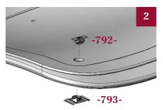
Stud retainer assembly includes upper Hold in place the lower clip retainer spring clip (AS-PN 150-792-000) and lower clip retainer (150-793-000).
