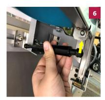
Attach new gas spring (extension end down as shown) to rear ball stud first, then locate close to front ball stud
