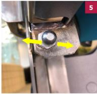
**Explanation:** the ball stud now has more dimensional play for attaching the new gas spring
