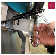
Tighten front ball stud using open end ½" inch wrenches. Cycle seat to verify functionality and adjust as necessary.
