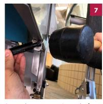
Secure the new gas spring to the front ball stud with a small rubber mallet
