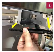
Remove gas spring from both seat frame ball studs
