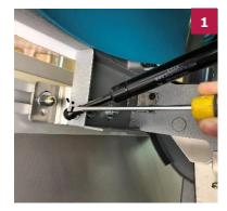
Flip-up seat and use a small flat head screwdriver (or similar tool) to pry off rear clip from gas spring
