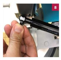
Attach front and rear spring clips to the new gas spring
