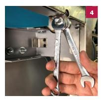
Loosen the front ball stud using two ½" inch open end wrenches
